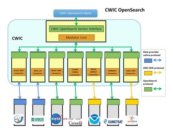
Fig. 2 The System Architecture of CWIC
