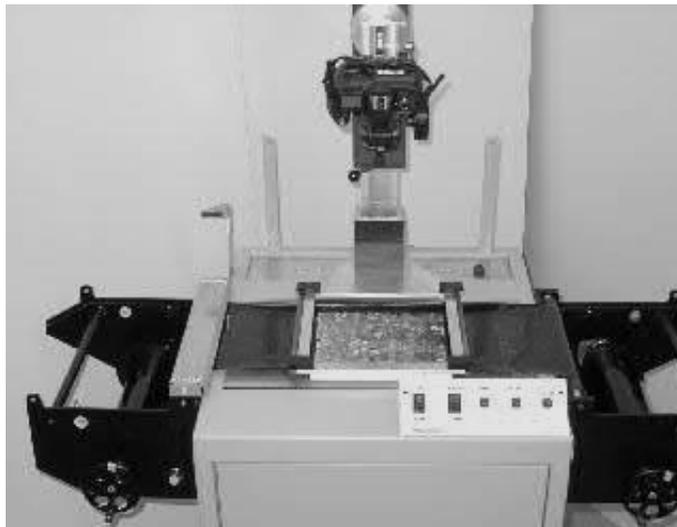
Fig. 2. Automated roll film digitization system
