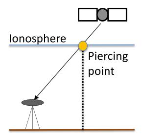
In this example: 1200 stations x 15 satellites generate a moving pattern of piercing points
