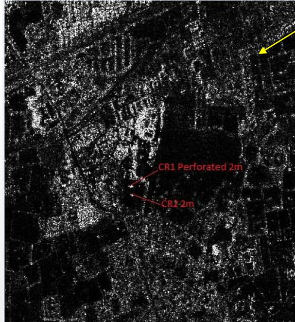
**Response of perforated CR in L-band airborne image of 14<sup>th</sup> February 2018**
