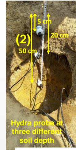
Hydra probe at three different soil depth
