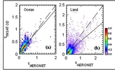
**Figure. (a) and (b)** Scatter plot of INSAT-3D & AERONET AOD over 5 ocean and 22 land sites, respectively. For land, the linear regression is  $\tau_{INSAT-3D} = 0.61\tau_{AERONET} + 0.07$  ( $r = 0.69, \sigma_r = 0.15$ ), while for ocean the linear regression is  $\tau_{INSAT-3D} = 0.87\tau_{AERONET} + 0.08$  ( $r = 0.77, \sigma_r =$ ).
