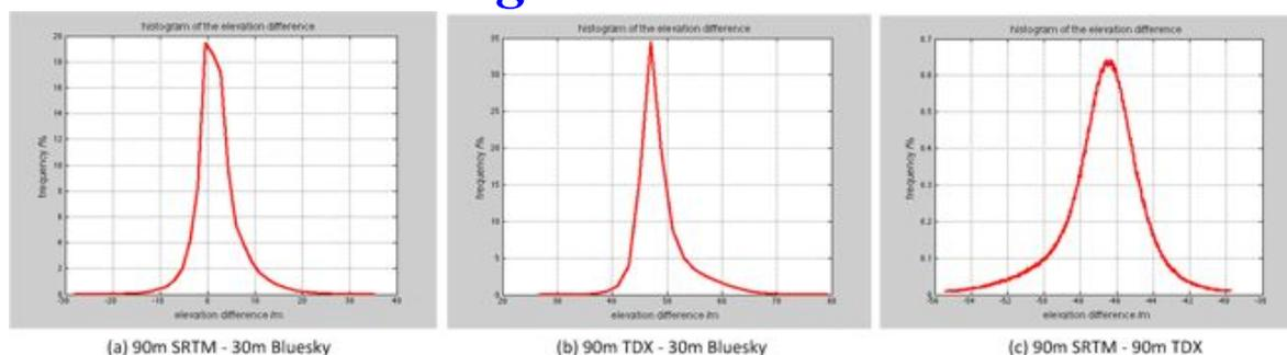
**Histograms of height difference between 90m SRTM-C DEM, 90m TDX IDEM and 30m BlueSky DTM**
