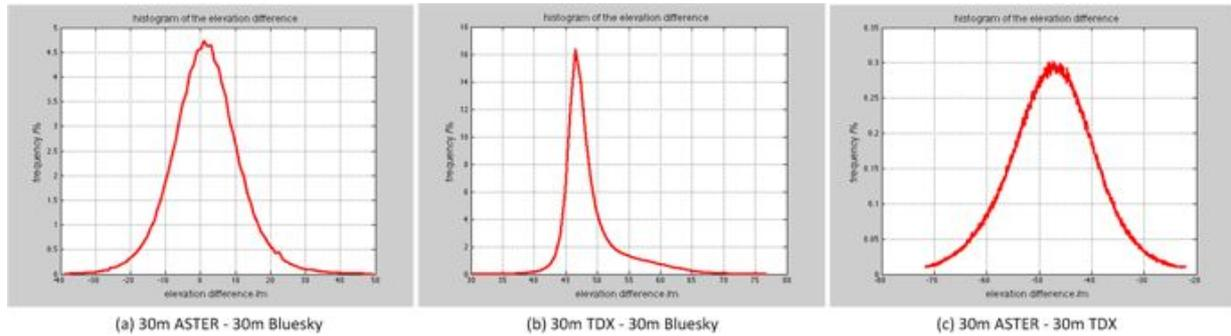
**Histograms of height difference between 30m ASTER GDEM, 30m TDX IDEM and 30m BlueSky DTM, all using the latter as reference DEM/DTM**
