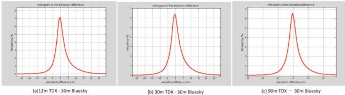
Histograms of height difference between 12m, 30m, 90m TDX and the reference BlueSky DTM
