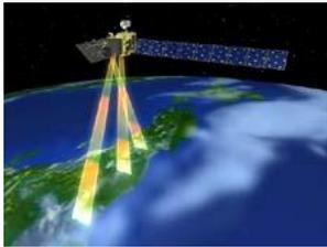
PRISM can acquire **triplet stereo** imageries by nadir-, forward-, and backward-radiometers with **2.5 m spatial resolution in 35 km swath**.
