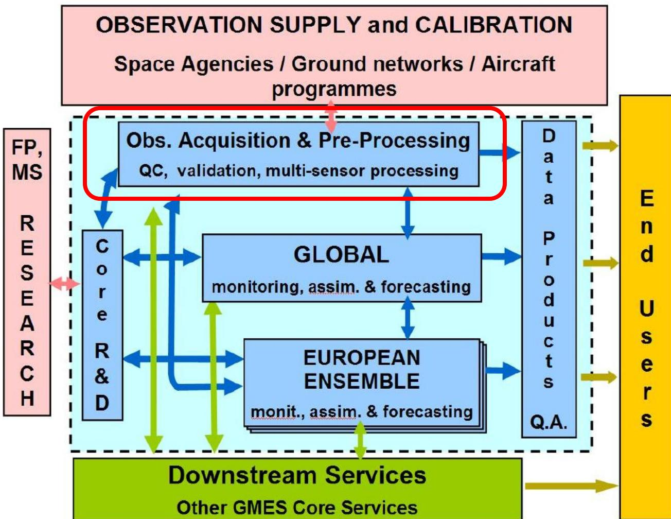
Figure 1: GAS functional architecture
