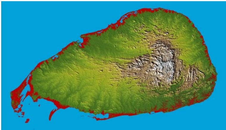
30m height "flood-fill" based on SRTM-DTED1@ 3" ( $\approx 90\text{m}$ )
