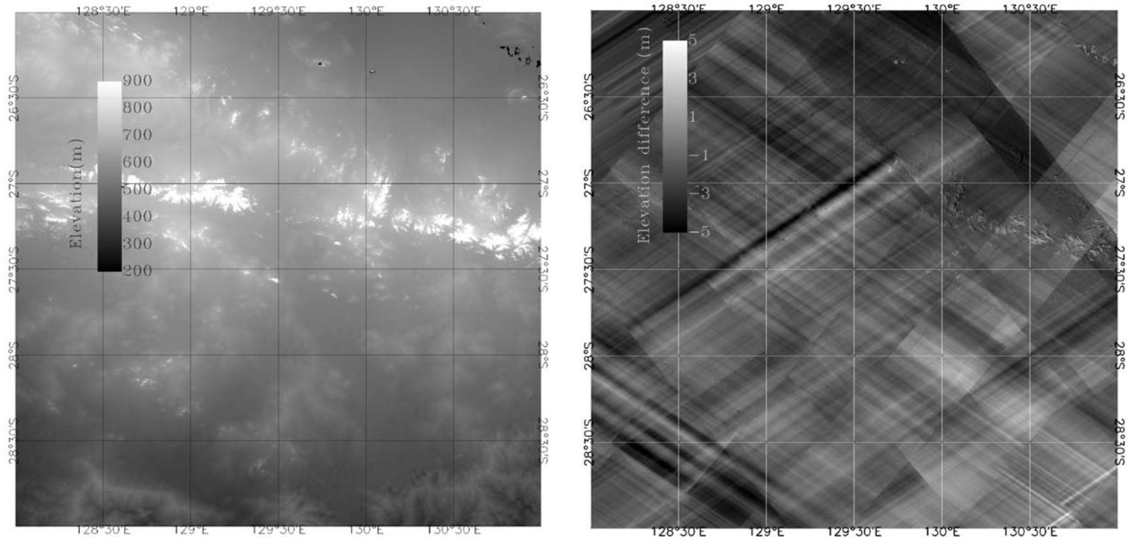
Left: New SRTM DEM over central Australia. Right: Correction (difference) between the new and original SRTM DEM. The crisscross pattern results from merging several SRTM ascending and descending passes containing artifacts. The ripples along each radar strip are removed with our new approach incorporating ICESat/GLAS data.
