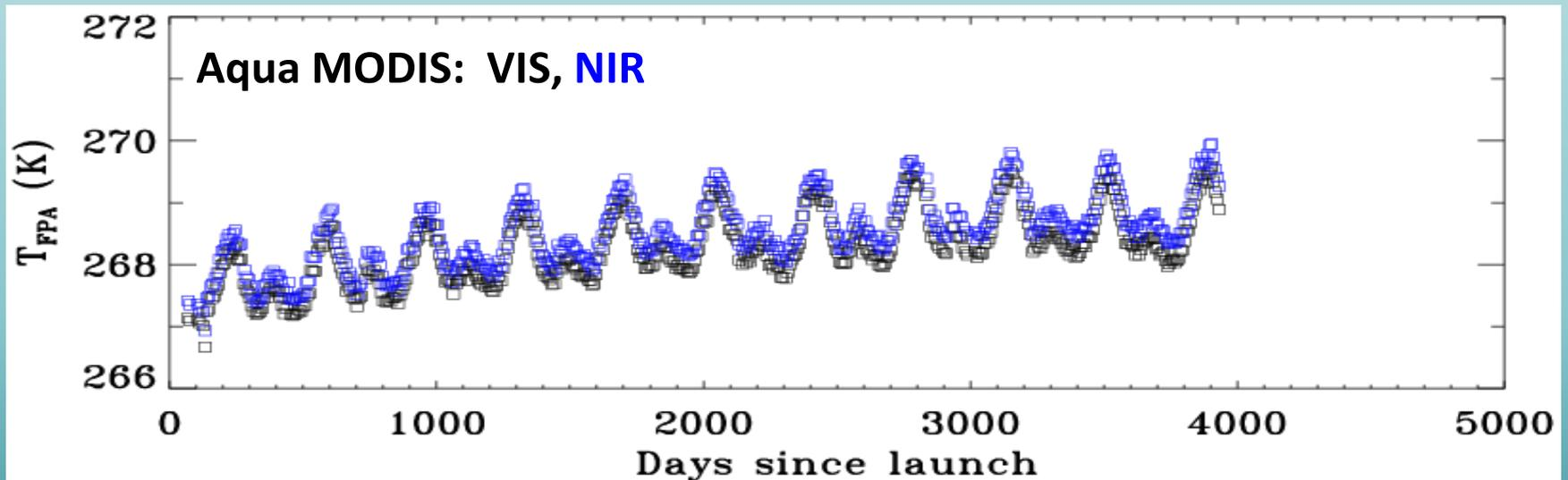
VIS & NIR FPA temperatures: similar to instrument temperatures
