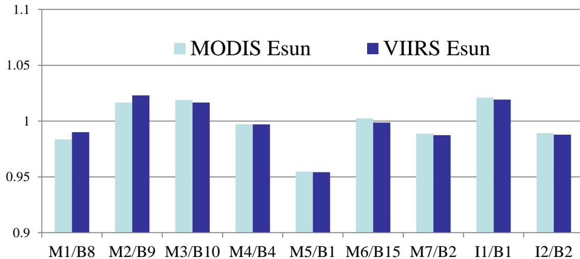
**VIIRS to MODIS radiance ratios determined using sensor RSR and Esun models for their spectrally matched bands**
