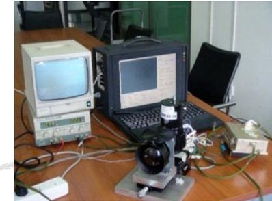
CH<sub>4</sub> leak imaging test
