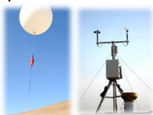
Radiosounding balloon Automatic weather station
