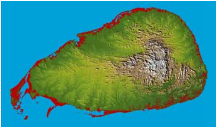
30m height “flood-fill” based on SRTM-DTED1® 3” (≈90m)
