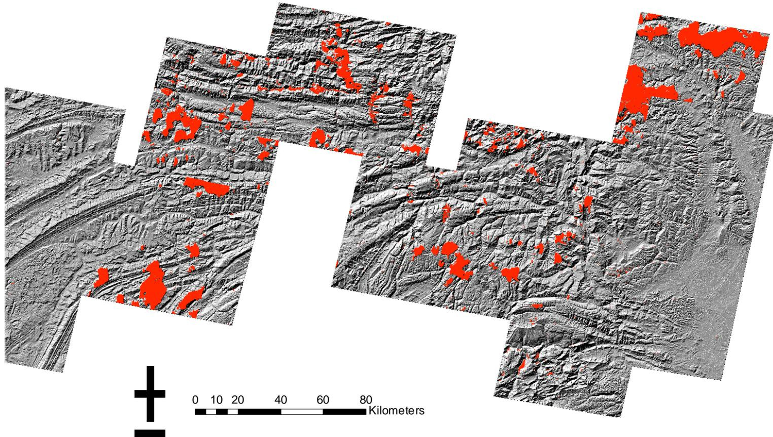
Elevation difference map created in ArcMap showing cloud cover artefacts in the ASTER DEMs. The map was obtained by subtracting the SRTM DEM mosaic from the ASTER DEM mosaic, removing subtle differences between the DEMs and applying a mask. The red areas represent height differences caused by clouds in the original ASTER L1a stereo images
