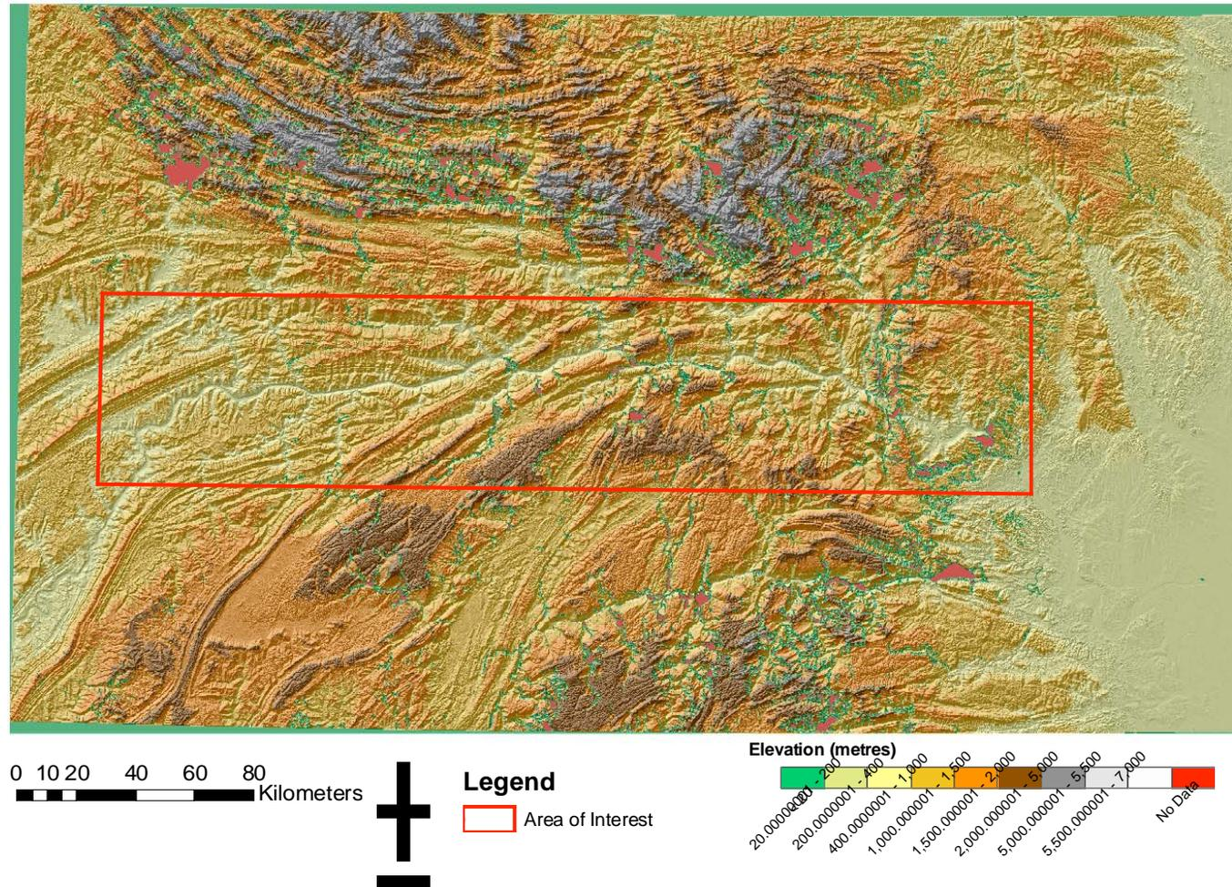
SRTM DEM mosaic hill-shaded in ArcMap with 30° altitude and 330° azimuth for the light direction and using ICEDS custom hill-shading colour scheme. Notice the red areas of missing data.
