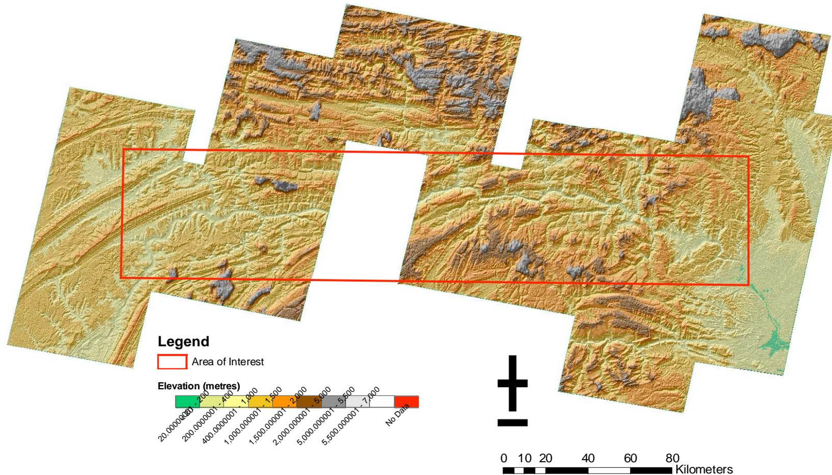
ASTER DEM mosaic hill-shaded in ArcMap with 30° altitude and 330° azimuth for the light direction and using the ICEDS custom hill-shading colour scheme. Note the grey areas which appear to be clouds.
