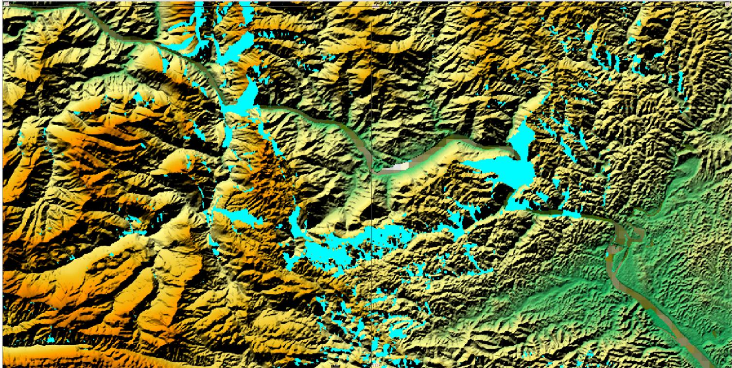
SRTM version 2 (so-called “finished”) DTED1 at 3” ( $\approx 90\text{m}$ )
