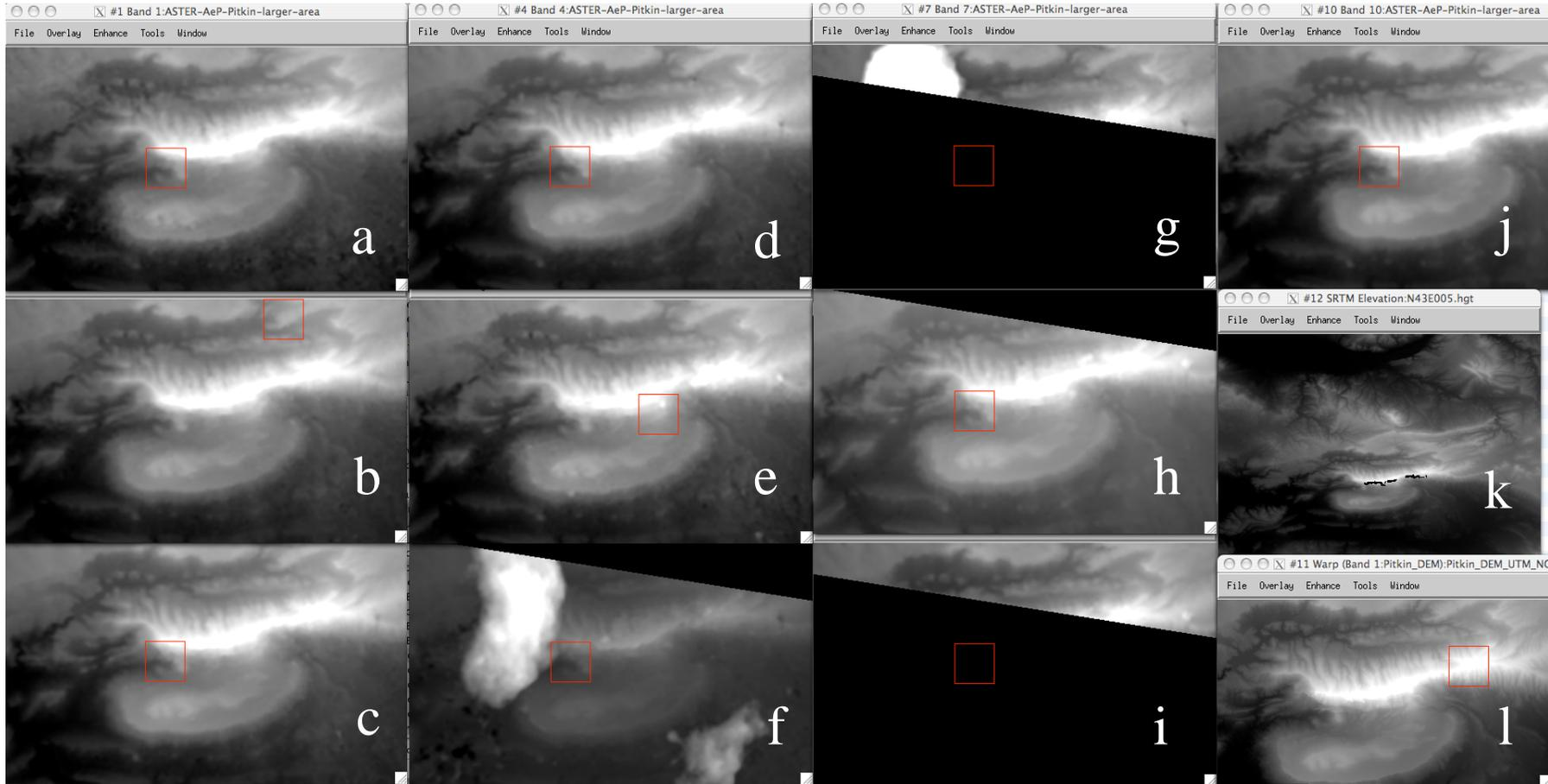
Note the clouds in (f) & (g), the missing areas in ASTER in (f-i). (k) shows SRTM ( $\approx 90\text{m}$ ) and (l) ground truth DEM ( $Z_{\text{rms}}=1.3\text{m}$ )
