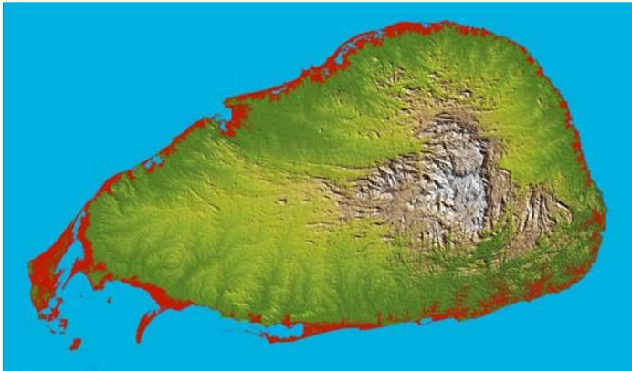
30m height “flood-fill” based on SRTM-DTED1® 3” (≈90m)
