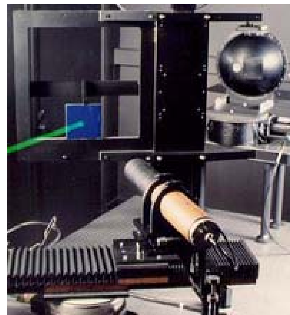
Photo of Spectral Tri-function Automated Reference Reflectometer (STARR)
