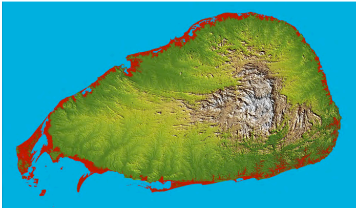
30m height "flood-fill" based on SRTM 3" (~90m)
