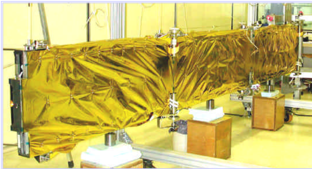
Arm deployment demonstration for planarity calibration measurements. (EADS-CASA courtesy)
