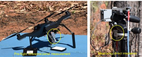
Drone based spectral data collection trial over Litchfield site synchronous with a Sentinel-2a overpass as a preparatory exercise for Phase 2
