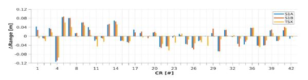
Figure 23: Average range offset for the individual CRs computed from range residuals of the experimentally calibrated Sentinel-1 IW data (see Table 8) and the TerraSAR-X ScanSar data (range results of Figure 13).
