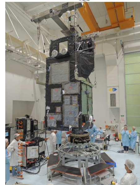
Sentinel-3B during the Rockot Launcher Fit Check Test
