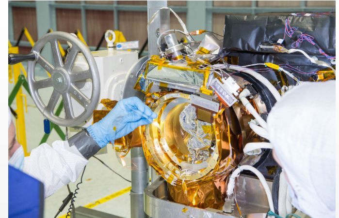
Shimming the TIRS-2 Focal Plane
