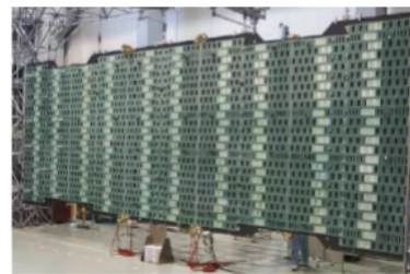
PALSAR-3 antenna PFS tests
