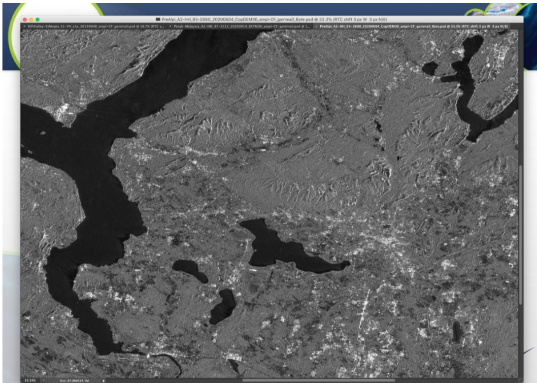
Radiometric Terrain Correction (RTC) – 3 pixels shift N and E
