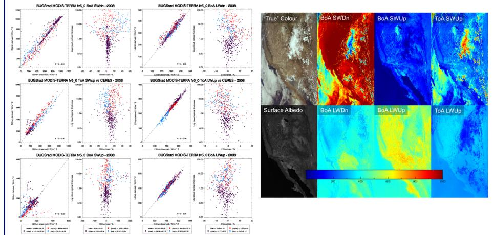
A recent addition to the ORAC suite is the ability to use the derived cloud and aerosol properties to calculate broad-band fluxes (shortwave, longwave, PAR) at TOA and BOA. The broadband radiative transfer is performed using either the BUGSrad (Stevens et al., 2001) or Fu-Liou (1993) models. The radiative consistency from visible to thermal IR provided by the ORAC algorithm is key to these calculations.
