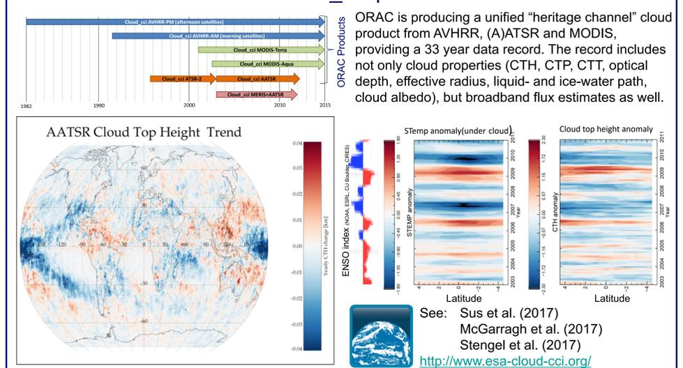
ORAC is producing a unified "heritage channel" cloud product from AVHRR, (A)ATSR and MODIS, providing a 33 year data record. The record includes not only cloud properties (CTH, CTP, CTT, optical depth, effective radius, liquid- and ice-water path, cloud albedo), but broadband flux estimates as well.
