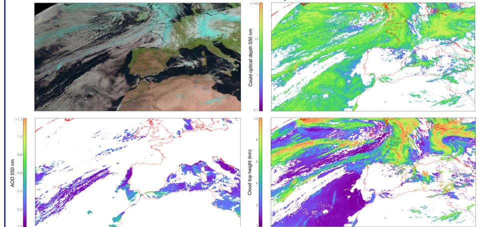
RAL has a prototype NRT processing system in place for SEVIRI, producing aerosol and cloud properties from 3-hourly EUMETCast imagery. Quicklook imagery is available from: <https://goo.gl/6fudaf>. The above scene, from 9:00 UTC, 26 July 2017, shows smoke plumes over the Mediterranean Sea and Atlantic from wild fires near Toulon and South of Lisbon.
