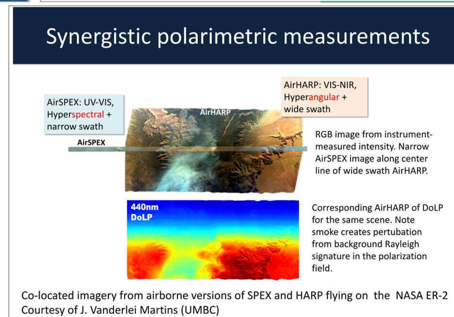
RGB image from instrument-measured intensity. Narrow AirSPEX image along center line of wide swath AirHARP.
