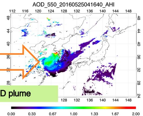
AHI IR cloud masking works successfully on GOCI AOD to filter out cirrus or shallow cloud contamination as retaining high AOD well.
