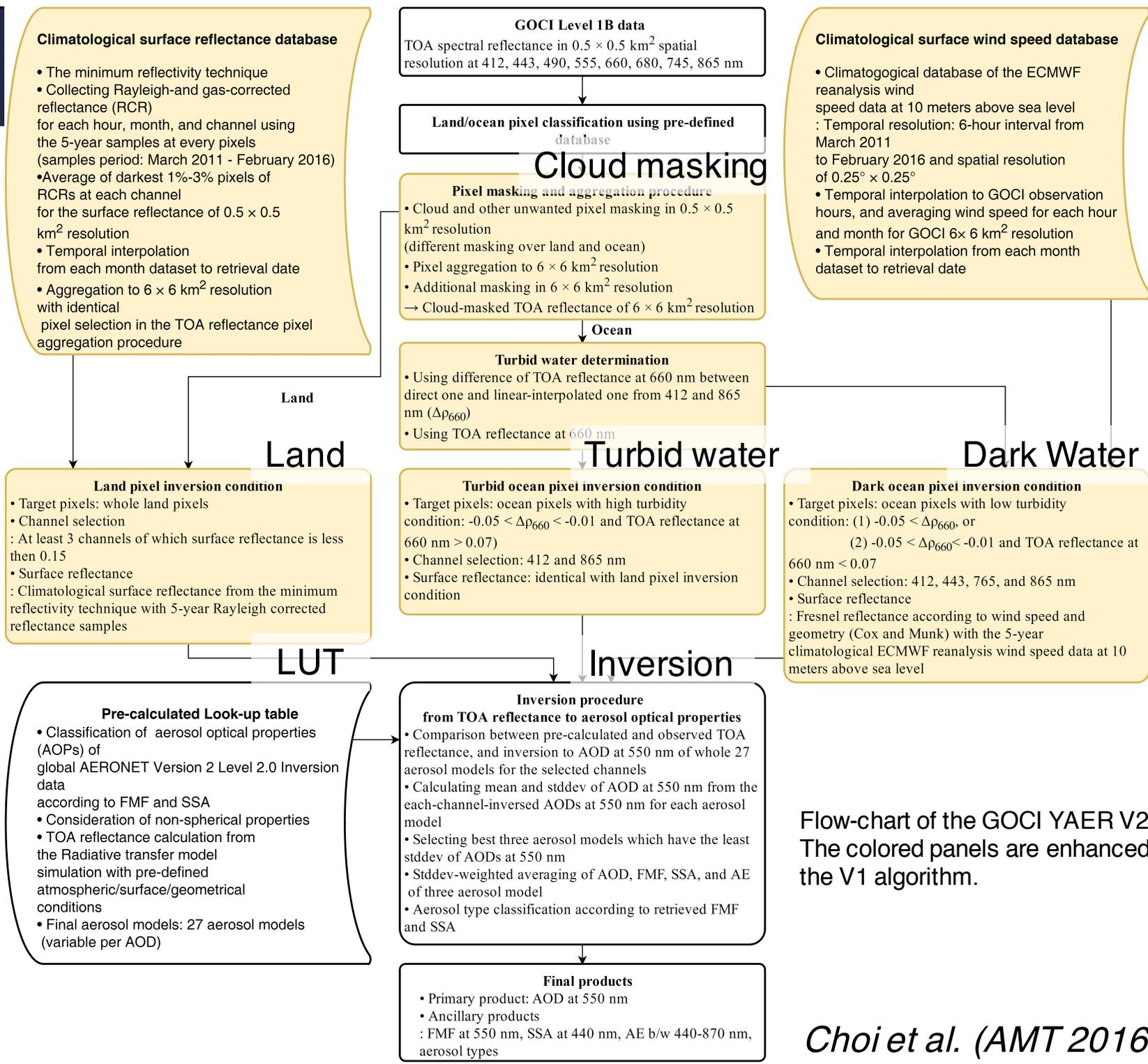
Flow-chart of the GOCI YAER V2 algorithm. The colored panels are enhanced parts from the V1 algorithm.
