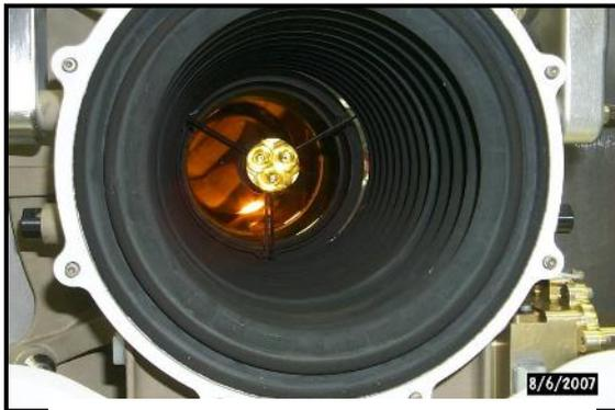
Telescope baffle assembly, showing lamps for flat fields
