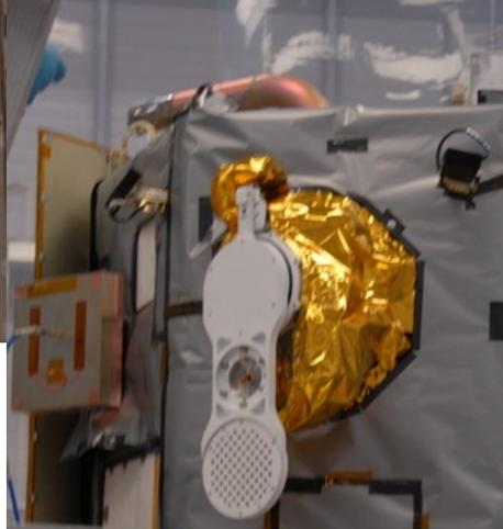
The on-board calibration (OBC) system consists of a rotating calibration paddle that carries:
