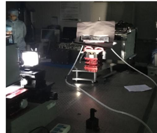
Put the known concentration of NO<sub>2</sub> into the cell, let light pass through it, then retrieve the observed spectrum, compare the retrieved results with NO<sub>2</sub> concentrations in the cell
