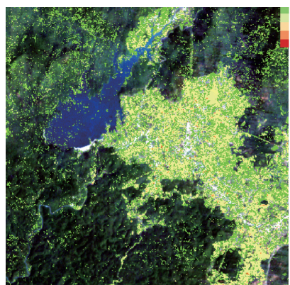
Land change detection results over Bediaye, Vietnam from 2000 to 2016. The product shows the number of land class changes over the time period. The region to the east of the lake is a new water dam project. Local decision-makers are able to use this information to track the progress of infrastructure development as well as identify remote regions of illegal deforestation.
