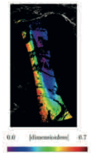
Figure 3.3 (after Meister et al., 2011) Degree of linear polarization (a dimensionless quantity from 0 to 1, where 0 is unpolarised light and 1 is completely linear polarised light) of the TOA radiances for an orbit of MODIS Aqua data over the Pacific Ocean for August 14, 2000. MODIS Aqua equator crossing time is 13:30; for a sensor with a noon crossing time a more symmetric distribution around nadir is expected.
