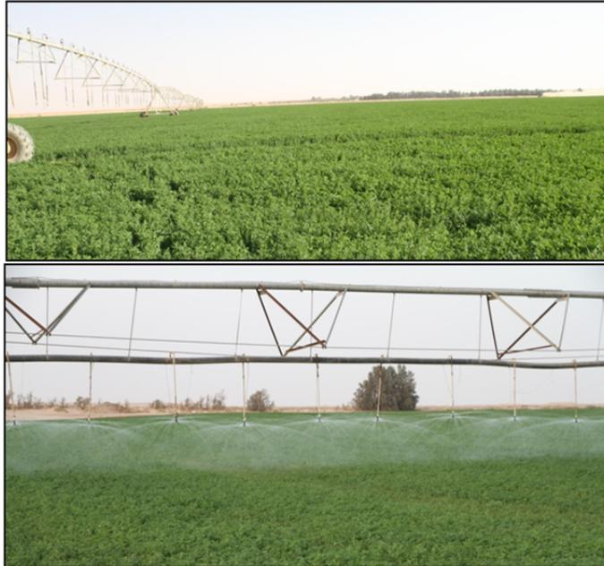
**Figure 92: Alfalfa Field under Centre Pivot Irrigation System**
