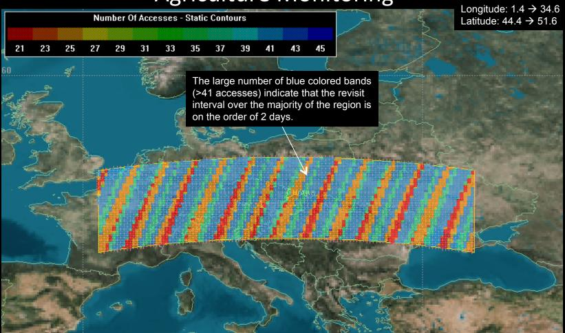
The picture shows the potential number of times LDCM and the Sentinel 2 satellites accessed areas on the ground over an 80 day period of time.
